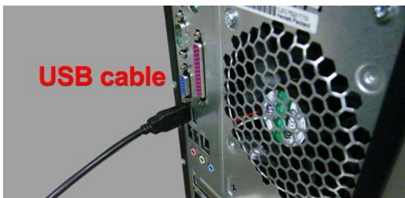
Computer rear side – USB cable connection
