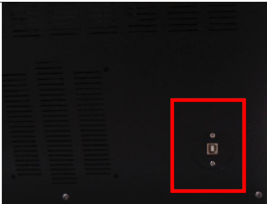
Darkroom back side– USB cable connection
