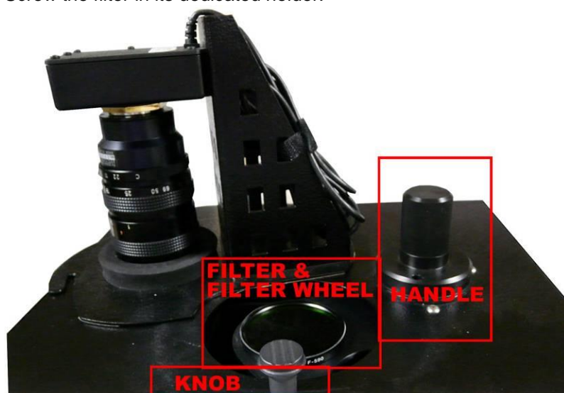
Figure 3: Top of the darkroom. The camera holder is positioned to facilitate the filter installation.
