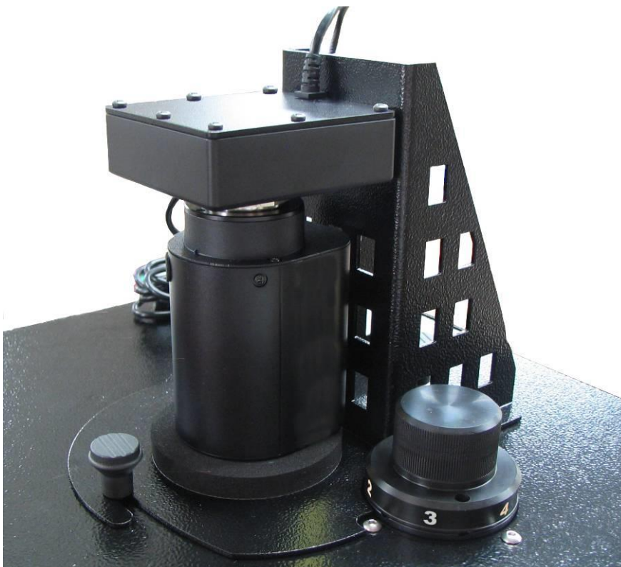
Illustration 3: the camera/optics installed on the top of the darkroom (front side)
